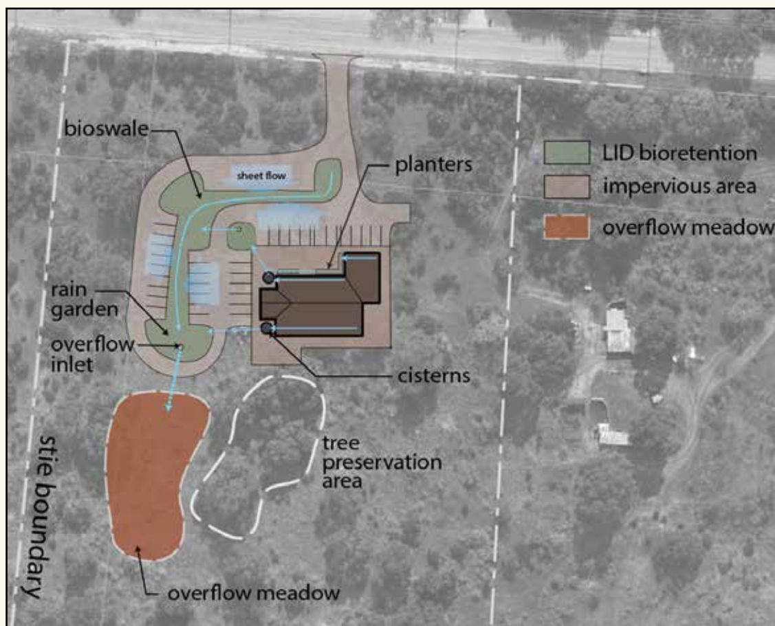
Figure 38. Site plan showing office development with LID. Blue arrows indicate general direction of flows. Dashed lines indicate pipes; solid lines are surface flows.
